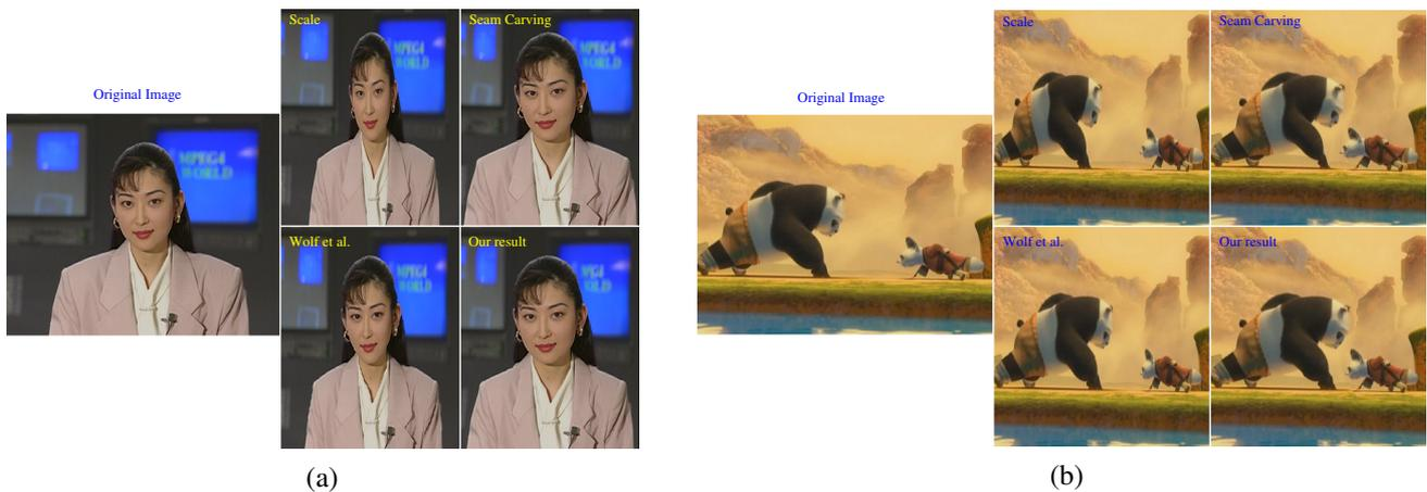
Fig. 11. Video retargeting results of (a) "Akiyo" and (b) "Kung Fu Panda". For both examples, the top-left images are the result of bicubic interpolation. The bottom-left images are the results of Wolf et al [1]. The image-based seam carving results are depicted in the top-right and the results of the proposed fast video carving algorithm are shown in the bottom-right.
