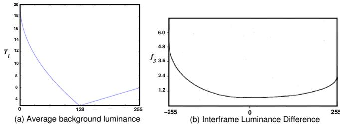
Fig. 6. (a) Illustration of luminance modeling.  $T_l$  is a function of average background luminance. (b) Temporal masking function.
