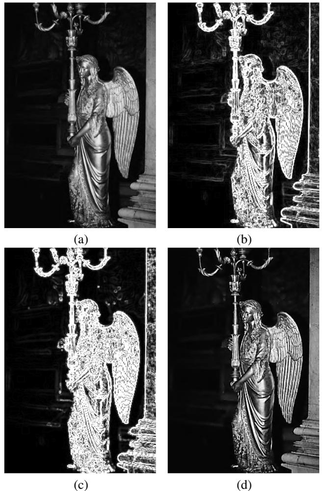
Fig. 5. (a) The source image. (b) The gradient map obtained by Sobel operator. (c) The energy map after applying JND-based importance enhancement scheme. (d) The enhanced image of (a).
