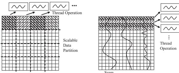
Fig. 8. Two types of parallelization operations: image convolution operation (left) and image resizing operation (right).
