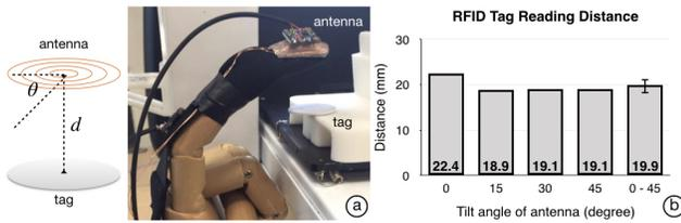
**Figure 3: Understanding the tag reading range of the customized antenna: (a) experimental apparatus; (b) results.**
