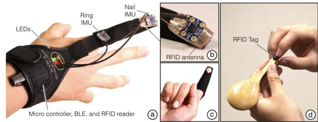
**Figure 2: Hardware prototype: (a) overview. (b) nail-mounted RFID antenna and an IMU; (c) the exposed fingertip; (d) example object (spoon) with an RFID tag attached.**
