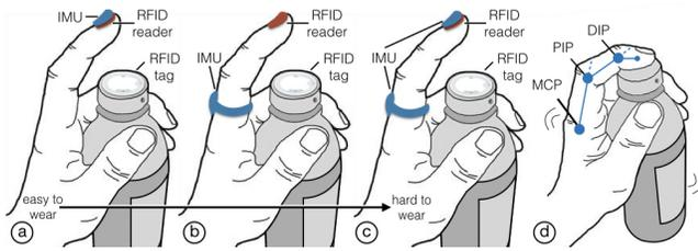
**Figure 1: Finger-worn RFID motion-tracking devices in three different IMU configurations with an RFID antenna placed on the nail: (a) NailOnly: only one IMU on the nail; (b) RingOnly: only one IMU on the ring; (c) Nail+Ring: one IMU on the nail and another IMU on the ring; (d) an example of the use of the index finger joints.**
