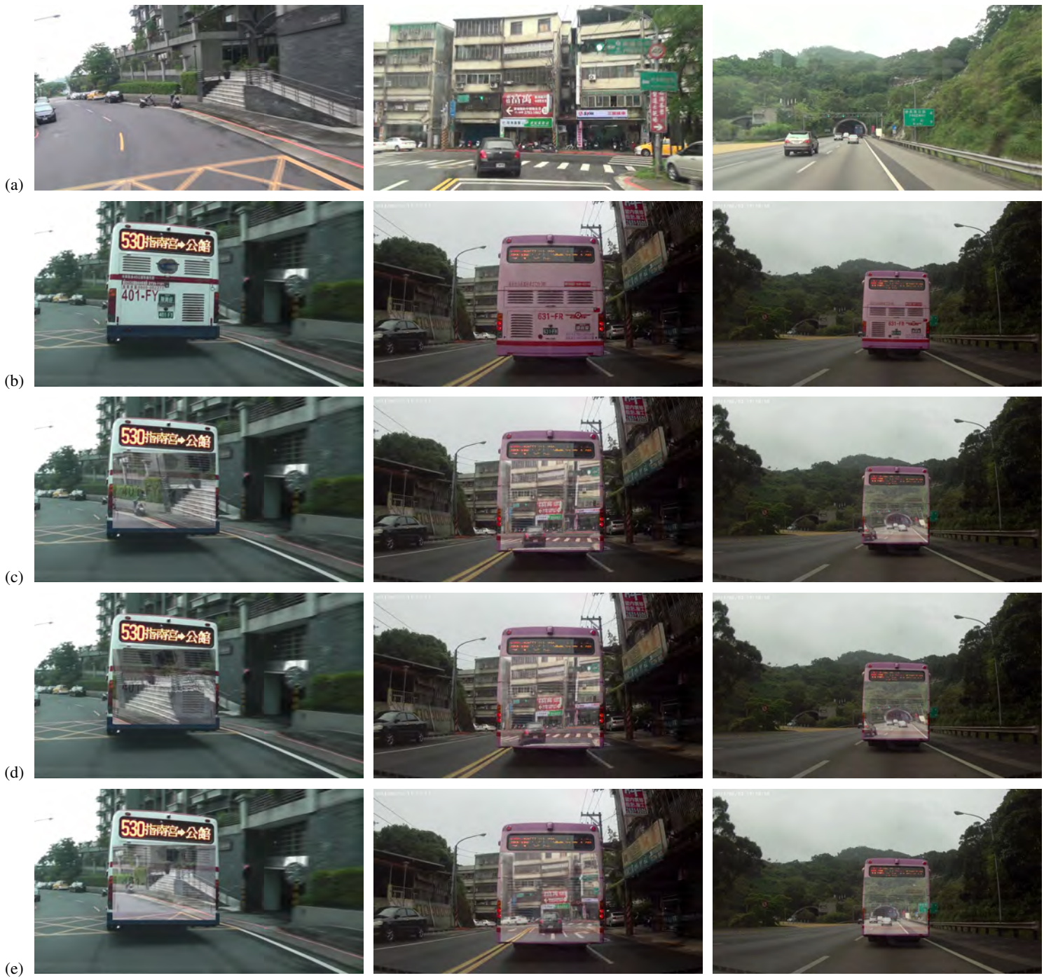
Figure 6: Qualitative comparisons. Challenging frames of reference sequence (a) and target sequence (b) are shown. (c) Aligned image using a global homography method. (d) Aligned image using Moving-DLT method [8]. (e) Aligned image with our method.
