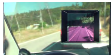
Figure 1: Previously proposed See-Through System (STS) presents to the driver a view with images taken from the preceding vehicle directly super-imposing over the image area occupied by the preceding vehicle [2]. However, the drivers need to pay extra attention since the perceived contextual information from different views are highly inconsistent.
