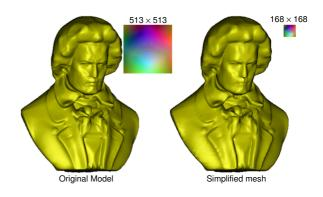
Fig. 1. Multi-resolution models by resizing geometry images. Left is the original 3D mesh with corresponding geometry image of size  $513 \times 513$ . The simplified 3D surface obtained by geometry image resizing to the size of  $168 \times 168$  is shown in the right side.
