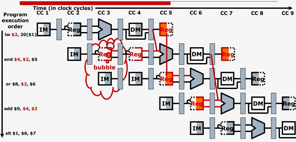
we can stall the pipeline by keeping an instruction in the same stage
