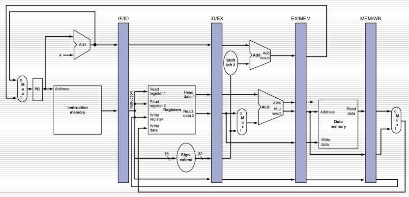
□ State of pipeline in a given cycle <sup>140</sup>
