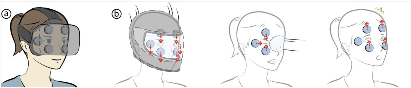
**Figure 1.** Masque is a prototype HMD integrating with six skin stretch modules. (a) Six shear factors are placed on the facial interface and can generate 2-degree-of-freedom lateral skin stretches, (b) which enables various skin stretch feedback or directional cues in virtual reality.
