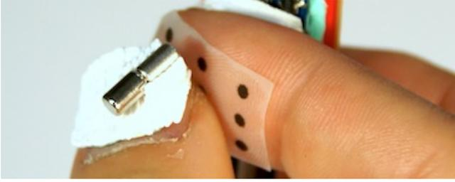
**Figure 5.** To guide the calibration, a translucent dot pattern is fixed to the index fingertip, thus helping to obtain good homographic transformations.
