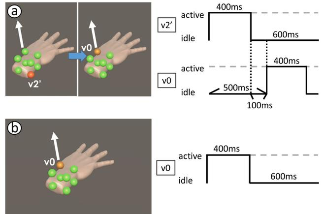
Figure 5: Illustration of directional feedback and active duration of motors. (a) Motion feedback (b) Point stimulus
