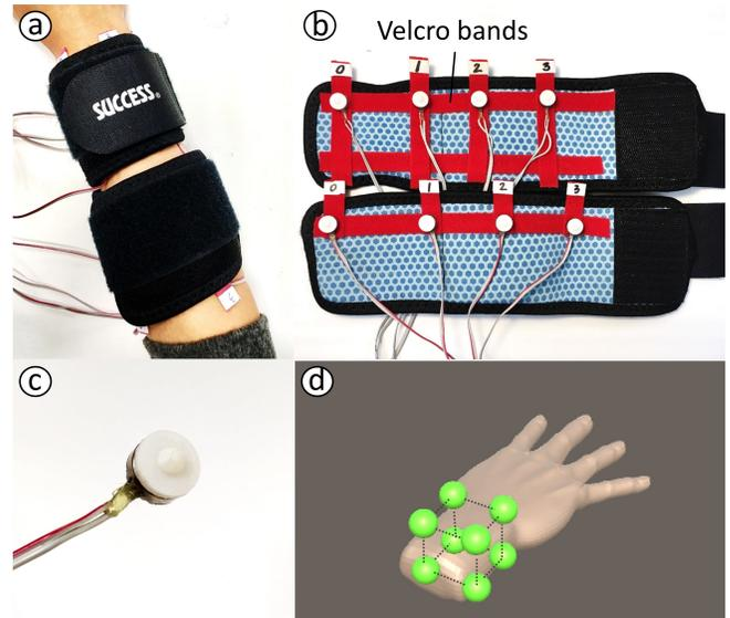
Figure 1: The devices and motors for our experiments. (a) The vibrotactile wristbands worn by a participant. (b) The details of vibrotactile wristbands and the arrangement of motors in the wristbands. (c) The motor with plastic caps. (d) The layout of 8 motors on the wrist. Each green sphere in the figure represents a vibration motor.
