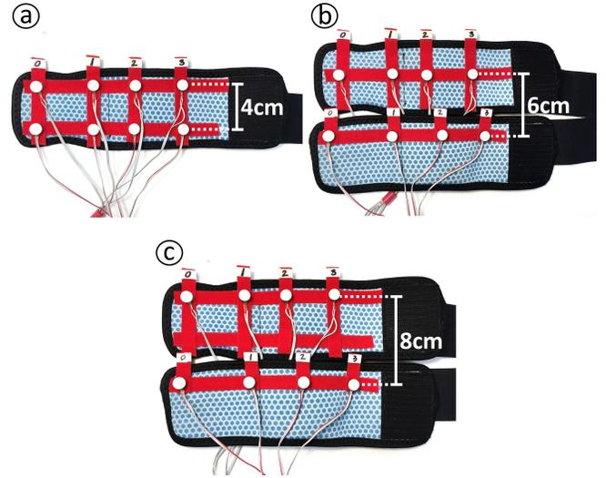
Figure 3: The arrangement of motors and the vibrotactile wristbands worn by the user. (a) The form of 4cm distance. (b) The form of 6cm distance. (c) The form of 8cm distance.
