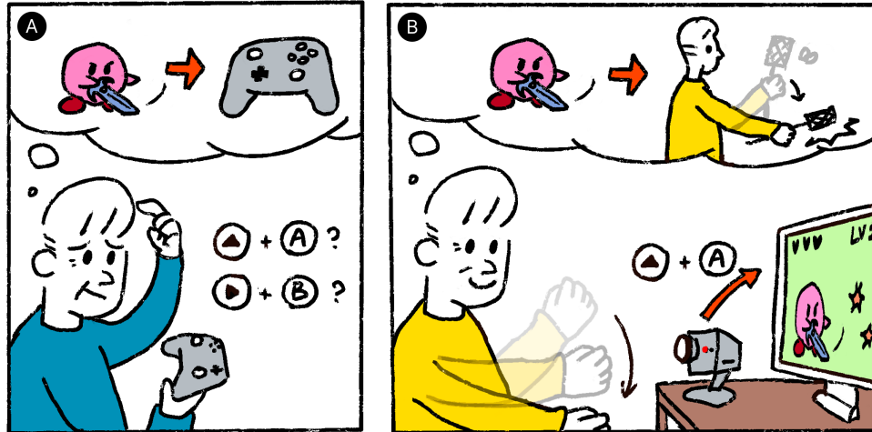
Figure 1: (A) Older adults often face difficulties with commercial games using standard controllers, as complex button mappings and fine motor demands hinder usability and engagement. (B) ElderPlay is a real-time game input translation system that enables gameplay through intuitive body movements without modifying the original game. It combines user-defined gesture input for expressive actions with conventional controls for movement, balancing accessibility and gameplay fidelity.
