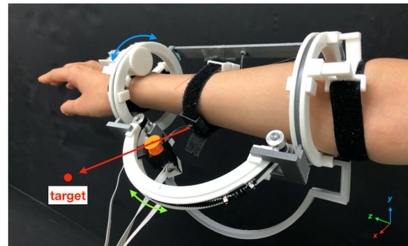
**Figure 1: GuideBand provides intuitive 3D multilevel force guidance by pulling the wristband toward the target direction.**
