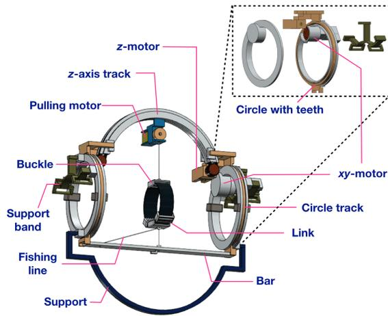
**Figure 2: The hardware structure of the GuideBand prototype.**
