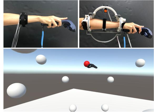
**Figure 7: Vibrotactile (upper-left) and force (upper-right) guidance wristbands. Lower: The scene in the guidance study with twenty balls. A ball turns red when touched by the controller.**
