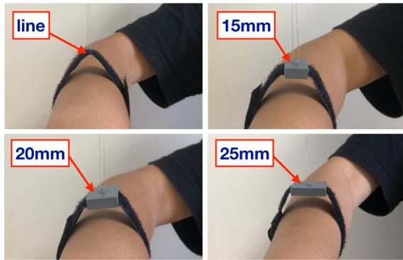
**Figure 3: Different buckle sizes to enhance the pulling force guidance.**
