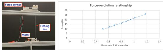
Figure 5: Pulling force stimuli measured by a force sensor.
