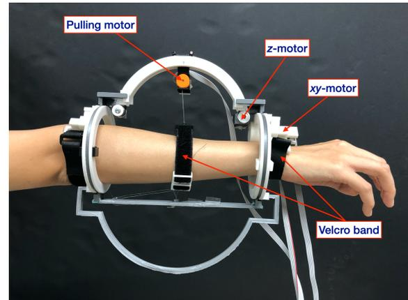
**Figure 4: GuideBand prototype worn on a forearm.**
