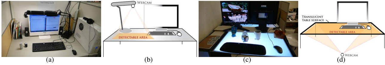
Figure 4. Two installation types. (a) & (b) Eagle-eye view installation. (c) & (d) Under-desk installation.
