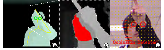
Figure 3: Occlusion-free eye-tracking. (a) The depth image and skeleton information are used to detect occlusion. (b) Selected pixels for calculating optical flow. (c) Result.
