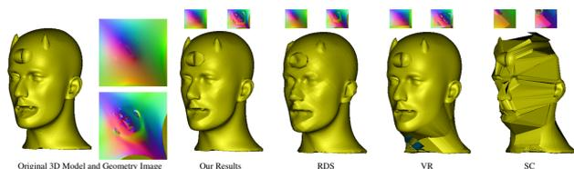
Fig. 7. Surface simplification of two example models by resizing the corresponding geometry images to the target sizes of  $105 \times 105$ .
