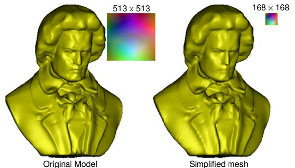
Fig. 1. Multi-resolution models by resizing geometry images. Left is the original 3D mesh with corresponding geometry image of size  $513 \times 513$ . The simplified 3D surface obtained by geometry image resizing to the size of  $168 \times 168$  is shown in the right side.
