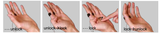
Figure 6: The process of gesture lock for palm-writing input. From left, the user performs palm-writing gesture (from unlock to lock state) to activate the interaction, and straighten the thumb (return to the unlock state) to finish interaction.
