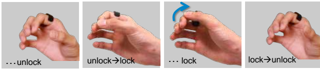
Figure 4: The process of gesture lock for on-finger pinch-and-slide input. From left, the user performs the interaction on the index finger (from unlock to lock state), and releases the pinch (return to unlock state).
