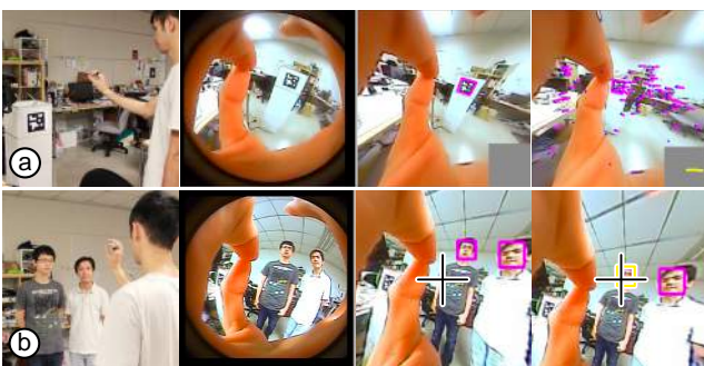
Figure 10: More context related functions can be incorporated with in-air pinch-and-motion input. (a) Direct interaction with a smart lamp through an AR tag. (b) Pick-and-drop information to a person via face detection.
