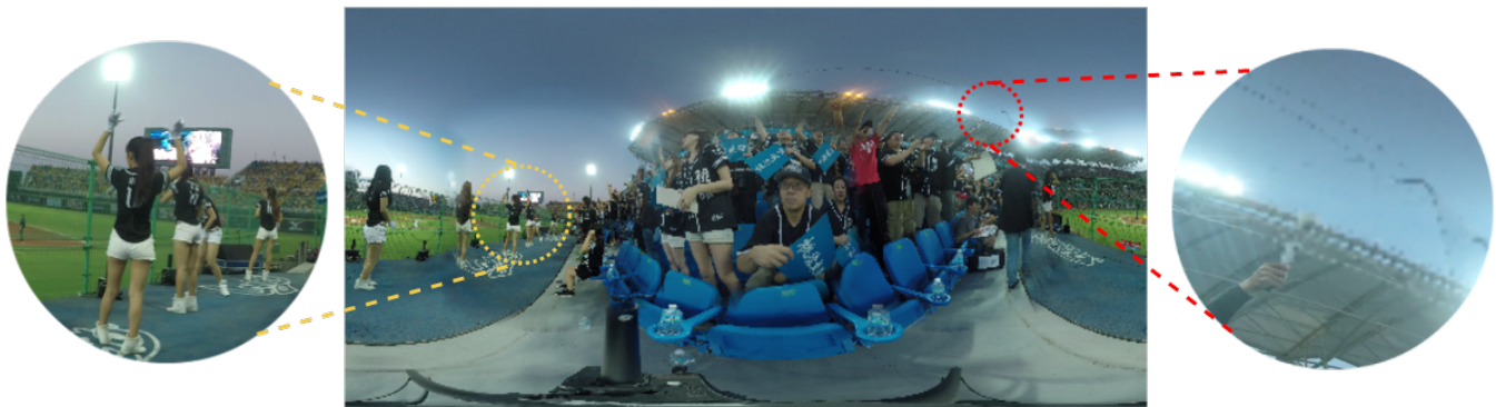
Figure 1: In this paper, we present a novel high-resolution video stitching framework for real-time VR. We adapt image resolution and level-of-detail by estimating foveal region. The yellow circle indicates a highly-salient region thus rendered in high resolution, while red circle indicates less important region thus rendered in low resolution. The proposed foveated stitching greatly reduces the number of pixels to be processed and overall graphics computation.
