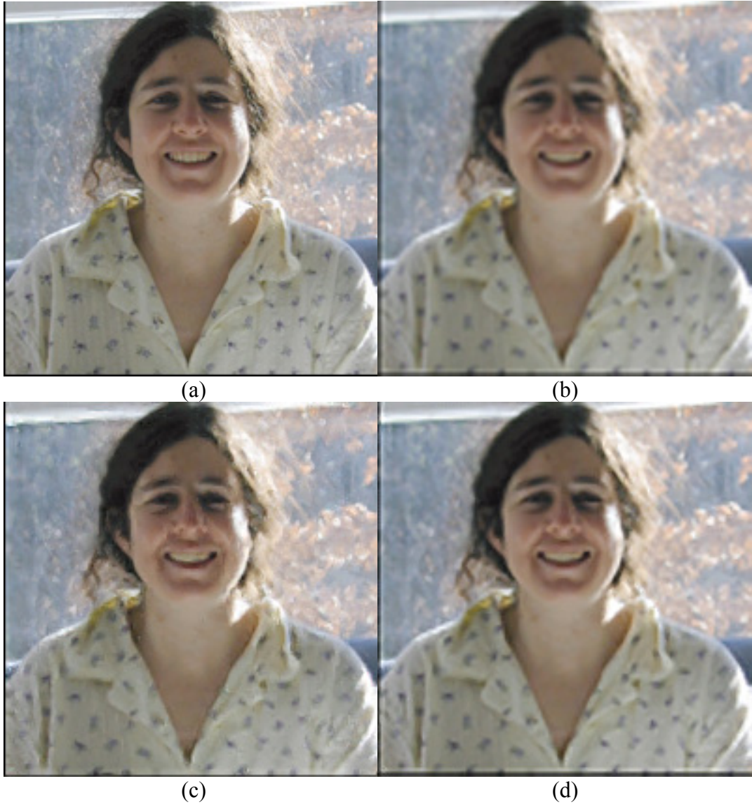
Fig. 6 The comparison of (a) ground truth image, (b) bi-cubic interpolation, (c) Freeman et al. 's method [3], and (d) our result.
