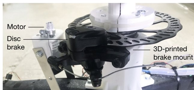
Figure 4: Disc brake modulating the resistive force of rotation.
